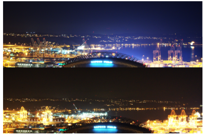
The photo above illustrates the light pollution caused by an HID system (top) compared to an LED system (bottom). (Photo courtesy of McKinsty)
